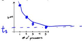
Find prediction rule  $H(p) = \frac{t_{NS}}{p} + t_{S}$  by minimizing MSE.  $= t_{NS} \left(\frac{1}{p}\right) + t_{S}$
