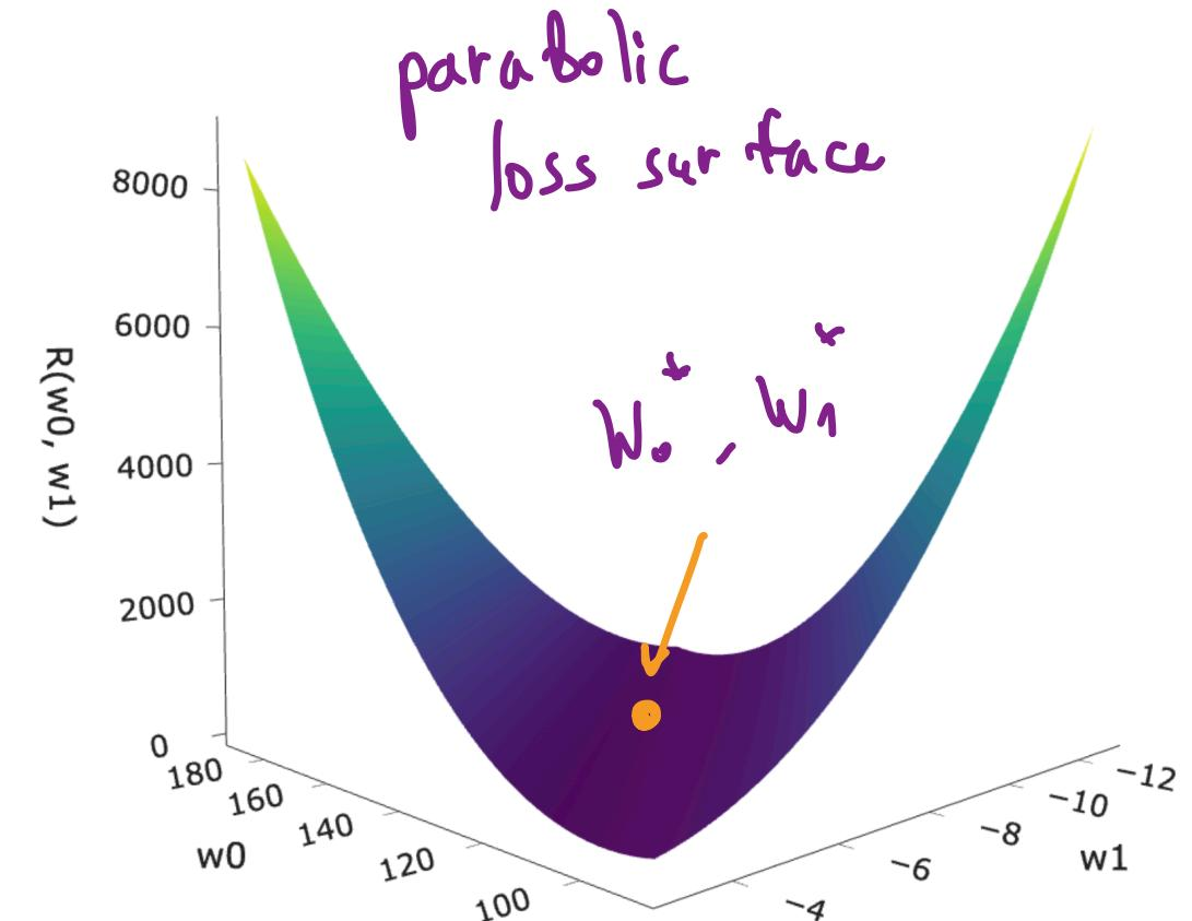
Minimizing mean squared error for the simple linear model
