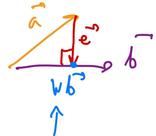
Projecting  $\vec{b}$  onto  $\text{span}(\vec{a})$
